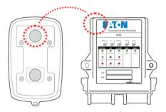
B. Adjust the positioning of the T110 magnet until the R260 (E-Stop) light begins to slowly alternate between GREEN and RED.
