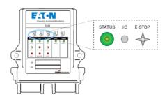
**Note:** If left idle in Setup Mode for over 30 seconds, the receiver will time out. The (Status) light and the (E-Stop) light will flash RED rapidly. To return to Setup Mode, repeat Step 3.
